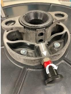
2.9 Release from the parking position and push down on the top plate until you hear a click indicating it is locked. Note: the red section should not be visible.
