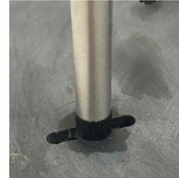
2.5 Ideally a snug fit over the rods is preferred, even if the rods lean inwards. This isn't an issue as there are rubber grommets at the base.
