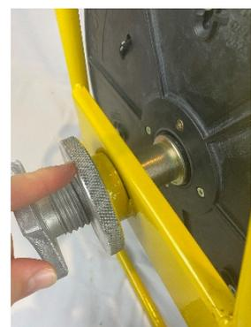
3.5 Locking pin – there are two locking pin positions to prevent the reel from moving before or after installation as a safety feature.
