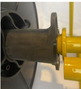
3.4 Feed the dispenser thread through the reel and hand tighten to the required tension. Complete locking the tension with the secondary knurled ring.
