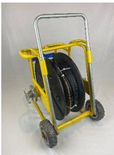
3.2 Before installation of the reel, ensure both payout arrows on the dispenser and the reel are in the same direction.
