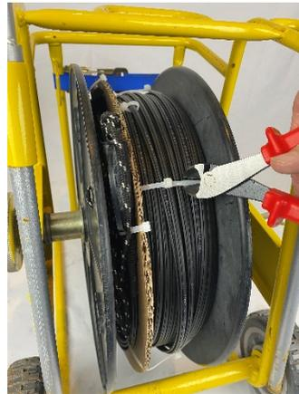
3.7 Normal usage of the dispenser is to feed the cable through the loop at the top; however, as the cable has a stop integrated on the coil to avoid the connector hitting the pulley, its preferred to feed the cable off the back of the drum to the pole.
