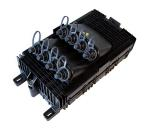
Mini-OTE 300-Series, Optical Terminal Enclosure, 8-port mini-size (DLX®) connector, with integrated 1x8 splitter, black, with grounding, external mounting. Splitter outputs connected to terminal housing ports, maximum 26 splices.
