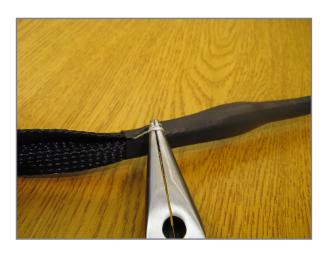
Pull out the rip cord to split the heat shrink along the path of the cord.
