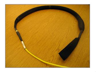
Remove the masking tape on the small end of the pulling sock.
