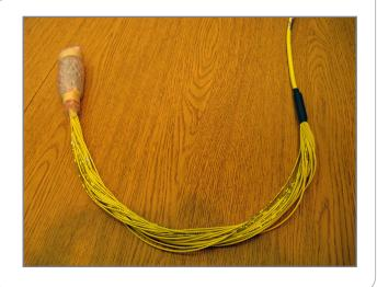
Remove the connectors from the plastic package, shown here at end of cable.
