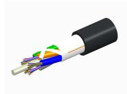
Fiber OSP cable, LightScope ZWP® Single Jacket All-Dielectric, 24 fiber, Gel-Free, Stranded Loose Tube, Singlemode G.652.D and G.657.Al, Meters jacket marking, Black jacket color
