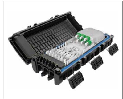
Fiber sealing closures need to accommodate a variety of cable sizes. But, historically they have been specific to a narrow range of cable diameters, meaning installers have to be trained to use many closure sealing types and to make sure that they stock the truck with the right products for the job. And when a cable is removed, the hole it leaves needs to be filled with a series of blank plugs, which are often misplaced.
