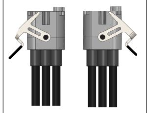
Align the hole of the latch arm with the hinge pin of the connector body and pull gently away from the body, just enough to clear the end of the hinge pin. Then pull the latch arm away parallel to the body
