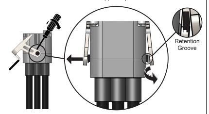
Once the latch is removed, bend the two arms back to 90° so they will fit tightly back onto the housing. To reattach, latch one arm over a hinge pin then roll other arm over the housing and onto the other hinge pin.
