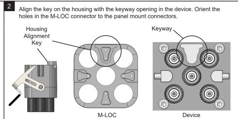
Align the M-LOC connector with the antenna mating interface and push firmly into place, eliminating gap between connector housing and bulkhead. While mating, a slight back and forth motion on the housing/cables will assist in centering and seating the port connectors into alignment. Push the latch toward the base of the antenna to engage the latch pins at the base of the connector housing.
