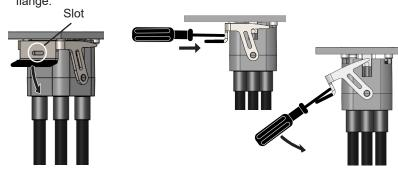
Grasp M-LOC connector housing, hold bent flange portion of latch back toward cable strain relief, pull the connector away from device. A slight back and forth motion on the housing helps to release the port connectors.
