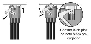
Apply force on the bent flange of the latch until the detents in the arms pop over the pins. There will be an audible and tactile click. To reduce hand strain, a screwdriver may
