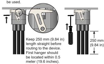
To remove the M-LOC connector pull latch flange away from the base of the antenna. To reduce hand strain, a flat blade screwdriver may be inserted in the slot above the latch flange and pulled down against the flange.
