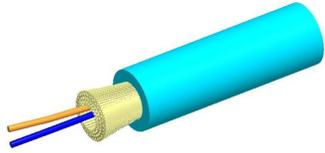
Fiber Indoor Cable, LazrSPEED® Low Smoke Zero Halogen Light Duty Interconnect, 2 fiber, Multimode OM4, Gel-free, Meters jacket marking, Aqua jacket color
