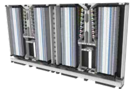
Figure 6: Cross Connect Four-frame block, deployed side-by-side, with side panels and with overlength storage bay in between the two twin frames. Recommended patch cord length for the cross connects between the two twin frames is 10 meters (34 ft).
