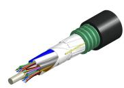
Fiber indoor/outdoor cable, LazrSPEED®, Single Jacket/Single Armor, 90 min Fire Survival, Low Smoke Zero Halogen (LSZH), 36 fiber, Multimode OM4, Gel-Filled, Stranded Loose Tube, Black jacket color, Meters cable marking
