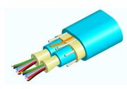
Fiber indoor cable, LazrSPEED® Low Smoke Zero Halogen Riser MPO Trunk, 16 fiber with 8 fiber 2.0mm subunits, Gel-free, Multimode OM4, Feet jacket marking, Aqua jacket color, B2ca flame rating
