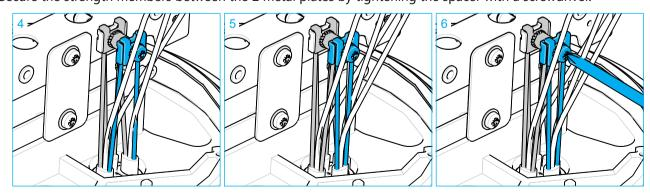
4 Attach another set of strength member plates onto the spacer using a screw with retaining washer. Secure the back
