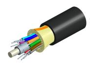
Fiber Indoor/Outdoor cable, TeraSPEED® Plenum Distribution, 18 fiber single-unit, Singlemode G.652.D and G.657.A1, Gel-free, Feet jacket marking, black jacket color
