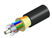
Fiber indoor/outdoor cable LazrSPEED® Indoor/Outdoor Plenum Distribution, 8 fiber single-unit, Multimode OM4, Gel-free, Feet jacket marking, Black jacket color
