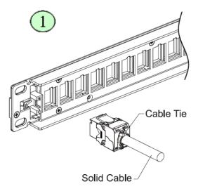
> Terminate cable on each RJ45 jack.
