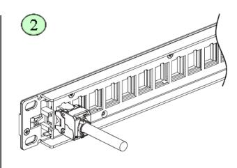
> Locate the RJ45 jacks into the panel.
