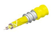
Fiber indoor cable, TeraSPEED® Plenum MPO Trunk, interlocking aluminum armored with plenum jacket, Singlemode G.652.D and G.657. Al, 96 fiber multi-unit with 12 fiber subunits, Yellow jacket color, Feet cable marking
