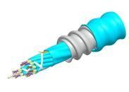
Fiber indoor cable, LazrSPEED® Riser/LSZH rated, MPO Trunk, interlocking aluminum armored, Multimode OM4, 12 fiber, Gel-free, Feet jacket marking, Aqua jacket color
