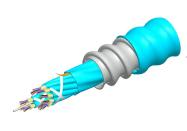
Fiber indoor cable, LazrSPEED® Riser/LSZH rated, MPO Trunk, interlocking aluminum armored, Multimode OM4, 144 fiber multi-unit with 12 fiber subunits, Gel-free, Feet jacket marking, Aqua jacket color
