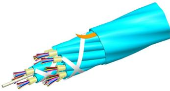
Fiber indoor cable, LazrSPEED® Plenum MPO Trunk, 64 fiber multi-unit with 8 fiber subunits, Multimode OM4, Gel-free, Feet jacket marking, Aqua jacket color
