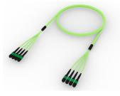
Ultra Low Loss (ULL) OM5 MPO16 (Pinned) to MPO16 (Pinned), Fiber Trunk Cable Assembly, 64-Fiber, Dual Rated (OFNR/LSZH)
