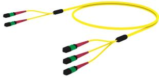
Ultra Low Loss (ULL) Singlemode G.657.A2, 2X3, MPO24 (Non-Pinned) to MPO24 (Non-Pinned-QSFP), 48-Fiber, Conversion Array, Plenum
