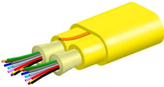
Fiber indoor cable, Plenum MPO Trunk Cable, 48 fiber with 24-fiber, 3.0 mm subunits, Gel-free, Singlemode G.657.A2/B2, Feet jacket marking, Yellow jacket color
