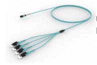
Ultra Low Loss (ULL) OM4 MPO8 APC (Pinned) to LC/UPC Uniboot, Fiber Array Cable Assembly, 8-Fiber, Dual Rated (OFNR/LSZH)
