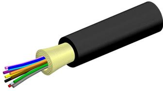
Fiber Indoor/Outdoor cable, Low Smoke Zero Halogen Micro Distribution, 24-Fiber, Singlemode G.657.A2, Feet jacket marking, Black jacket color, Dca flame rating
