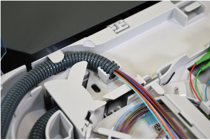
7.4. Push the flex tube in the flex tube holder. Feed the 900µm fibers towards the splice/patch area.
