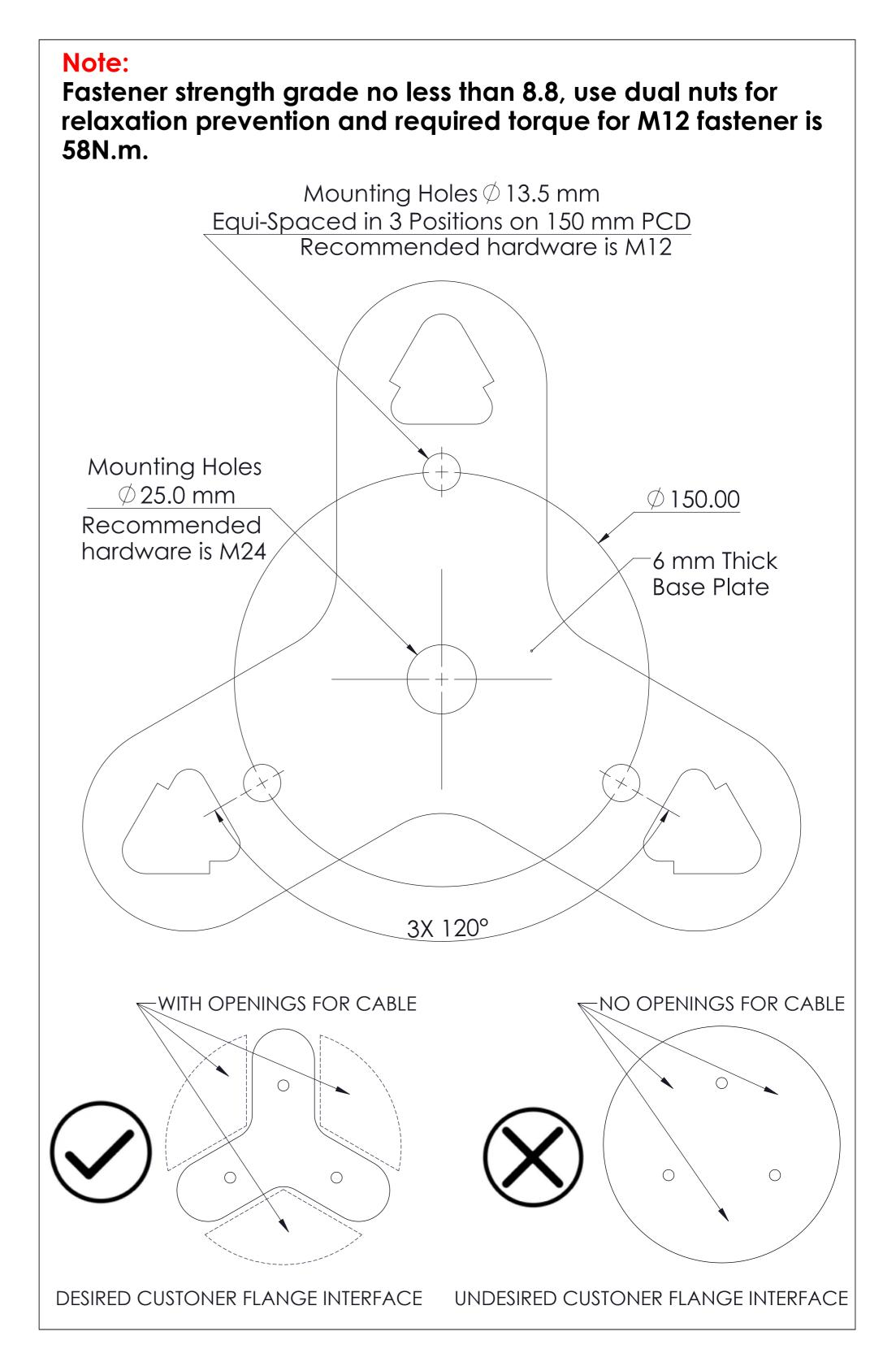
Figure 2. Mounting Holes on Base Plate Viewed From Bottom Side of Antenna
