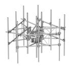
G23RHDX Monopole Sector Frame with spine extension for RRU Mounting,  $10.5 \, \text{ft} \times 2.88 \, \text{in} \, \text{OD}$  face pipes, includes nine  $2.88 \, \text{OD} \times 120 \, \text{in}$  antenna pipes
