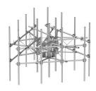
G23RHDX Monopole Sector Frame with spine extension for RRU Mounting, 12.5 ft x 2.88 in OD face pipes, includes twelve 2.88 OD x 120 in antenna pipes
