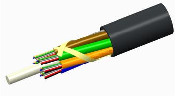
Fiber OSP cable, LightScope® ZWP Blown Micro Single Jacket, 24 fiber, All-Dielectric Stranded Loose Tube Arid-Core™ Construction, Gel-filled, Singlemode G.652.D and G.657.A1, Feet jacket marking, Black jacket color
