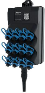
NOVUX™ Hardened Multi-fiber Terminal, 12 HMFOC ports, 2 fibers per port, Dielectric flat loose tube cable with HMFOC plug (female/no pin), 1500 ft/457 m, with universal mounting bracket
