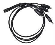
HELIAX® M-LOC Multiport cluster 4 ports SureFlex® cable assembly with Integrated Birdproofing Shell with interface type M-LOC latching male to 4.3-10 male with HELIAX® SureGuard weatherproofing on 4.3-10 end, size 1/4", length 3 meters,
