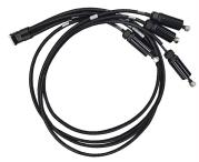
HELIAX® M-LOC Multiport cluster 4 ports SureFlex® cable assembly with Integrated Birdproofing Shell with interface type M-LOC latching male to 4.3-10 male with HELIAX® SureGuard weatherproofing on 4.3-10 end, size 1/4", length 5 meters,
