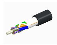
Fiber indoor/outdoor cable, LightSCOPE ZWP®, Single Jacket All-Dielectric, LSZH, 96 fiber, Gel-Free, Stranded Loose Tube, Singlemode G. 652.D and G.657.A1, Meters jacket marking, Black jacket color, Eca flame rating
