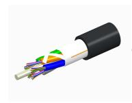
Fiber indoor/outdoor cable, LightSCOPE ZWP®, Single Jacket All-Dielectric, LSZH, 60 fiber, Gel-Free, Stranded Loose Tube, Singlemode G. 652.D and G.657.Al, Meters jacket marking, Black jacket color, Eca flame rating
