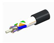
Fiber indoor/outdoor cable, Single Jacket All-Dielectric, LSZH, 36 fiber, Gel-Free, Stranded Loose Tube, Singlemode G.652.D and G.657.Al, Meters jacket marking, Black jacket color, Eca flame rating
