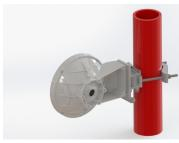
0.2 m | 0.67 ft ValuLine® High Performance Low Profile Antenna, single-polarized, 37.000 – 40.000 GHz, PBR320, polymer radome without flash, standard pack—one-piece reflector
