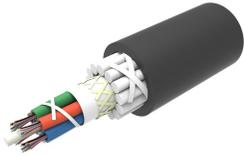
Fiber indoor/outdoor cable, TeraSPEED® Single Jacket/Single GRP Armor, Gel-filled, Stranded Loose Tube, Singlemode G.652.D and G.657.A1, Meters jacket marking, Black jacket color. Provides Rodent Resistance.
