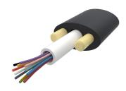
LightScope® ZWP Self-Supporting All-Dielectric Outdoor Drop Cable, 36 fiber Arid Core construction, central loose tube, no ripcords
