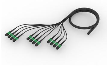
Ultra Low Loss (ULL) Singlemode, MPO12 Unpinned to Unconnectorized, Fiber Trunk Cable Assembly, 144-Fiber, Low Smoke Zero Halogen/Riser, Indoor/Outdoor
