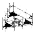
3-Sector Monopole Co-location Platform Kit, 30 in to 60 in OD, 14 ft 6 in face, includes twelve 126 in pipes
