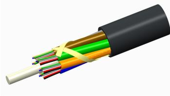
Fiber OSP cable, LightScope® ZWP Blown Micro Single Jacket All-Dielectric Outdoor Stranded Loose Tube Arid-Core™ Construction, 144 fiber, Singlemode G.657.A2, Gel-filled, Meters jacket marking, Black jacket color
