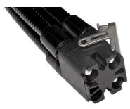
HELIAX® M-LOC Multiport cluster 4 ports SureFlex® cable assembly with interface type M-LOC latching male to N male,size 3/8", length 2.5 meters
