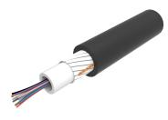
Indoor/Outdoor Low Smoke Zero Halogen, TeraSPEED® Central Loose Tube Fiber Optic Cable, 12-fiber, Singlemode OS2, Gel-filled, black. Provides Rodent Resistance.
