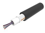
Indoor/Outdoor Low Smoke Zero Halogen, TeraSPEED® Central Loose Tube Fiber Optic Cable, 6-fiber, Singlemode OS2, Gel-filled, black. Provides Rodent Resistance.
