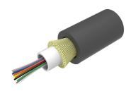
Indoor/Outdoor Low Smoke Zero Halogen, LazrSPEED® Central Loose Tube Fiber Optic Cable, 4-fiber, Multimode OM3, Gel-filled, black. Provides Rodent Resistance.
