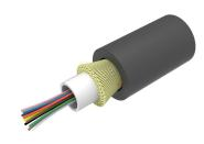
Indoor/Outdoor Low Smoke Zero Halogen, LazrSPEED® Central Loose Tube Fiber Optic Cable, 24-fiber, Multimode OM3, Gel-filled, black. Provides Rodent Resistance
