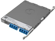
Propel ULL Singlemode MPO-08 front facing breakout module, 4 duplex LC/UPC to 1X8f MPO/APC pinned, Method B Enhanced
