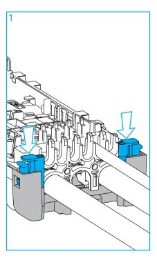
Position the organizer in the closure with the front side (drop side) facing on top. Push firmly on the snap features to lock the organizer in the closure. When a click sound is noticed, the organizer is properly locked.
