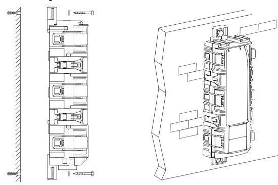
Using the mounting tabs as a template, mark the mounting screw locations on the selected surface for the installation. Install wall plugs first, then position the closure with the mounting tabs against the surface. Continue with the washers and the screws to secure the closure onto the surface.
