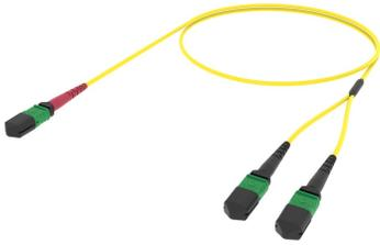
Ultra Low Loss (ULL) Singlemode, MPO/24(Unpinned) to MPO/12 (Unpinned), 24-Fiber, Plenum, Array Cord
