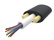
Fiber outdoor drop cable, LightScope® ZWP Self-Supporting All-Dielectric, Singlemode G.652.D and G.657.Al, 24 fiber, Arid Core construction, Gel-filled, central loose tube, no ripcords, Feet jacket marking, Black jacket color, 5000 ft
