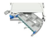
MFPS Fiber Optic panel, 1RU, 48 fibers/RU, splice/patch, SMOUV/front patch cords orientation to the left, 48 LC/UPC, OM4
