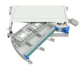
MFPS Fiber Optic panel, 1RU, 72 fibers/RU, splice/patch, SMOUV/front patch cords orientation to the right, 72 LC/UPC, OM4
